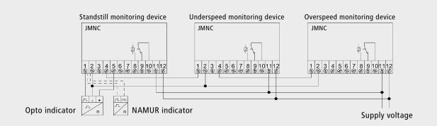
Example: Several rotational speed monitoring devices JMNC connected to one pulse indicator.
